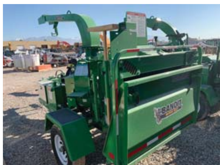
Chipper – Manufacturer: Bandit Model: 15XP Drum Style Brush Bandit 139 hp engine
